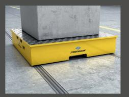
Height tolerance ±1 mm over a 5 m track, tolerance of the track gauge, ±0.5 mm
