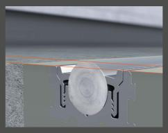
Tracks are protruding only a few millimeters above of the floor: 3 mm above ground level with RS25.
