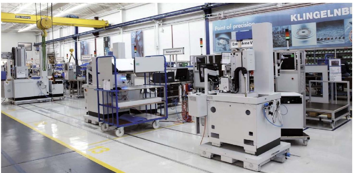
KLINGELNBERG converted from box to flow assembly. The decision for STROTHMANN RoundTracks® means that mobile shelves, for instance, can easily cross the line.
