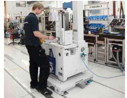
Mobile standing workplace with leveling platforms clearly visible in the floor.
