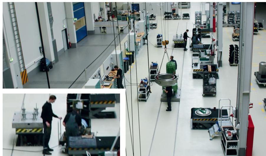
*The new production line consists of clearly defined stations and RoundTrack® floor rails that practically vanish in the hall floor. Lifting platforms integrated in the floor bring the assembly modules to an ergonomic height.*
