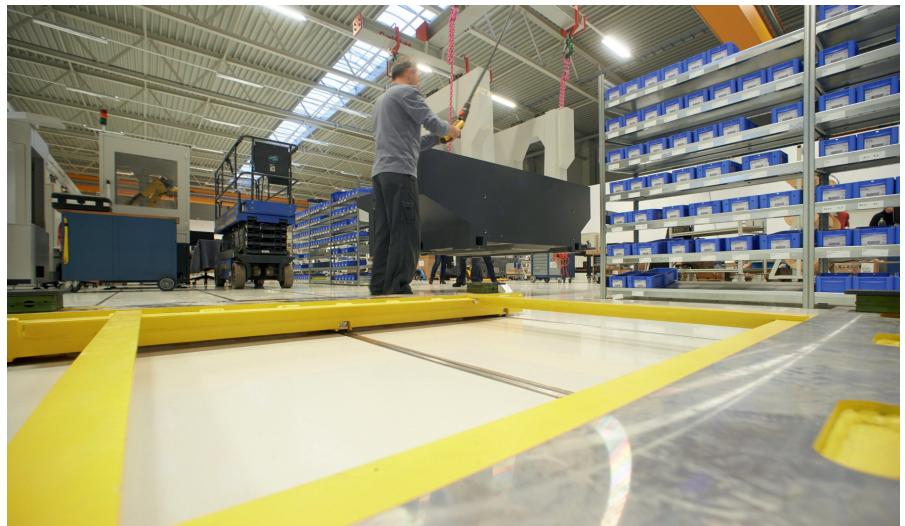
*RoundTrack®-Technology combines well with overhead cranes that are used to provide heavy parts and to transport finished units to the test field. Image: Kraas & Lachmann, Tübingen, Germany*
